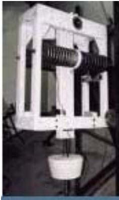
Figure 8: One of the TMDs designed for the skybridge legs of the Petronas Towers by RWDI Inc. (12 TMDs were installed three in each of the four legs)
