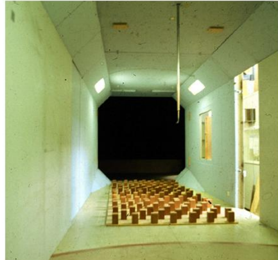
(A) 2m by 2m working section
